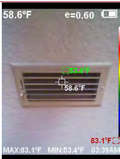
SHOWING SUPPLY VENT INFRARED TEMPERATURE SCAN.
