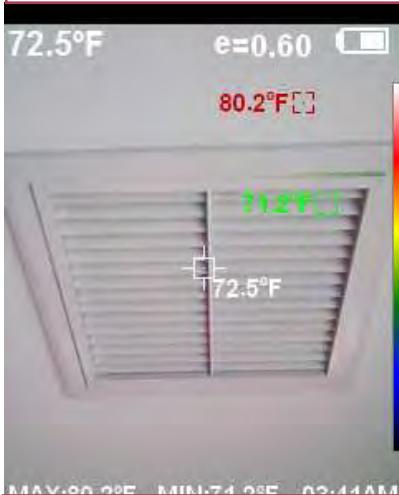
SHOWING RETURN VENT 2 INFRARED TEMPERATURE SCAN.
