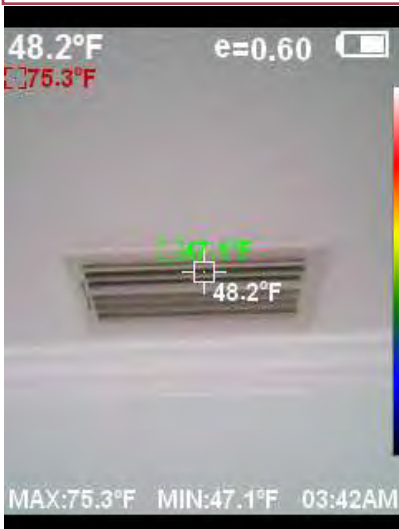
SHOWING SUPPLY VENT 2 INFRARED TEMPERATURE SCAN.
