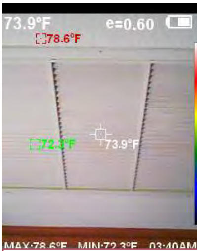
SHOWING RETURN VENT INFRARED TEMPERATURE SCAN
